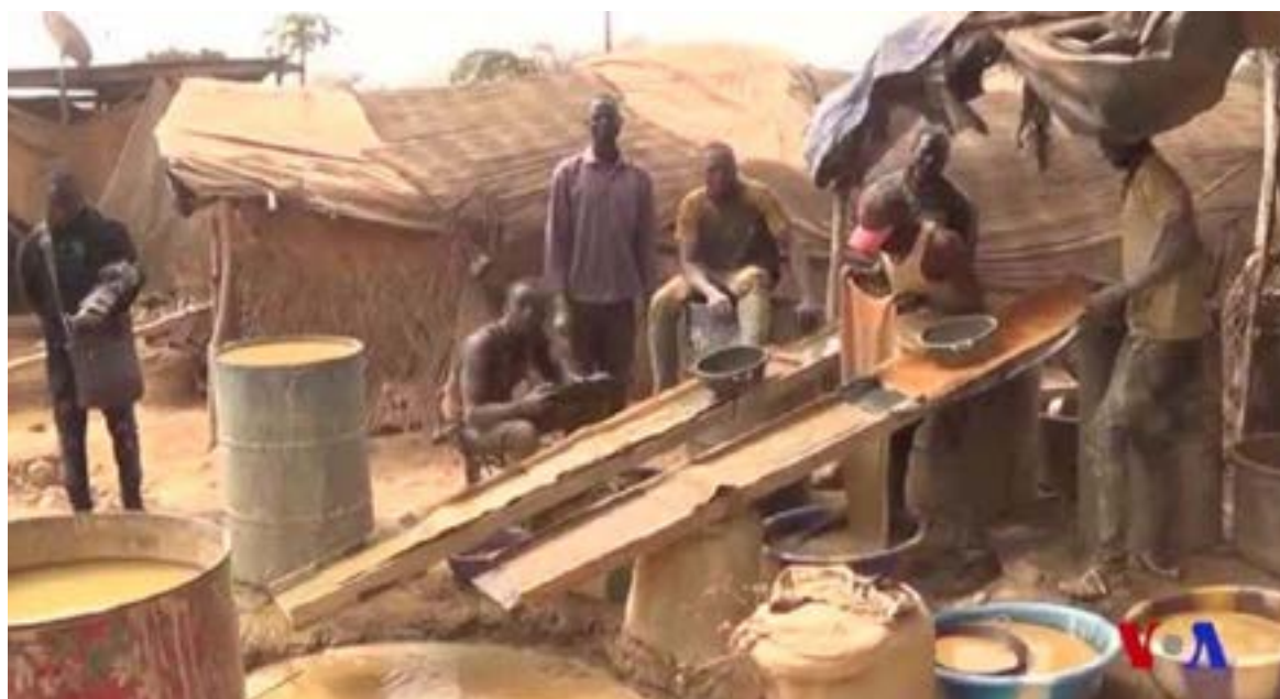
Figure 2 – Washing ore at the Bontcholi gold mine
