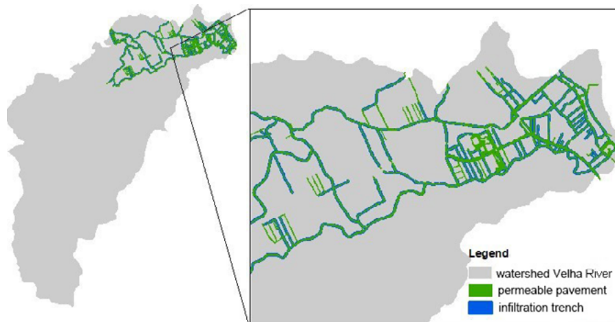
Figure 4 | Representation of areas with proposed incorporation of SUDS (permeable pavement and infiltration trench) in public areas of non-motorized mobility and rolling lanes of motorized mobility routes
