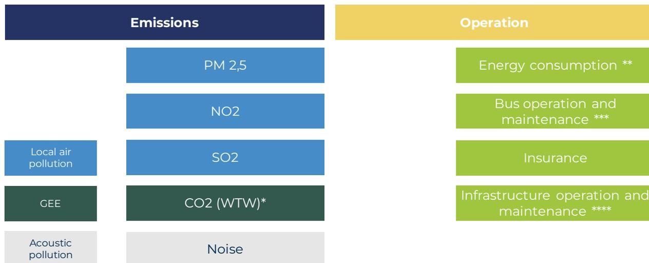
\*Well-to-Wheel: analysis that evaluates the total energy consumed by the vehicle for each kWh of energy or liters of diesel supplied to the vehicle's wheels, including all the steps covered by the well-to-wheel conversion, and, later, by the tank-to-wheel conversion.
